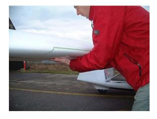
Always support the wing with flat hands on the lower surface, level with the spar (the thickest part of the wing) or at either end of the wing. Avoid putting pressure on the upper surface, as it is not reinforced.
