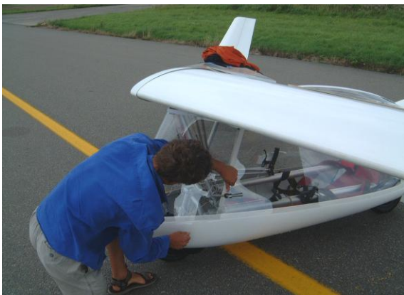
13. Go up the upright tube pressing the Velcro firmly in.
