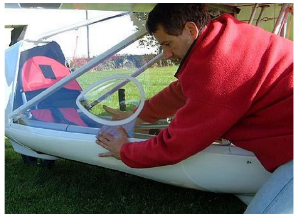
8. Make sure that the Velcro is properly in by squeezing tightly.
