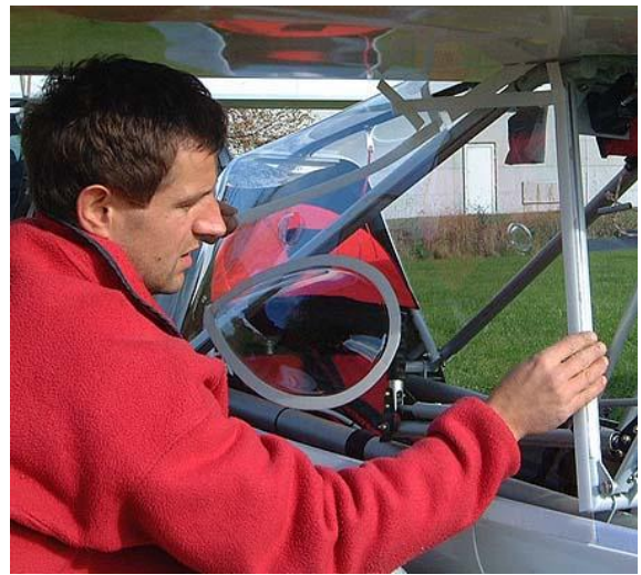
6. Follow the vertical edge engaging the Velcro.
