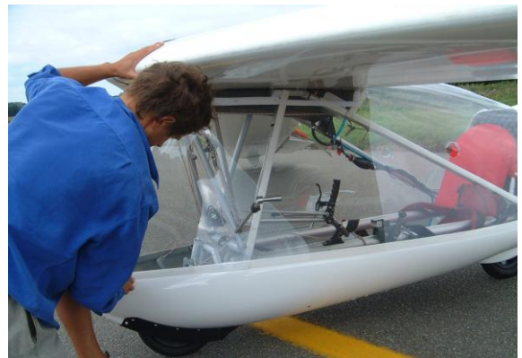
14. Go again along the fairing pressing firmly the Velcro in.
