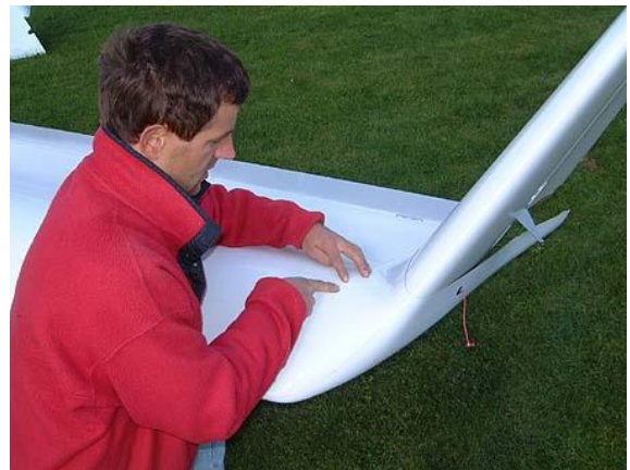
14. Press down to engage the Velcro from the line up point ...
