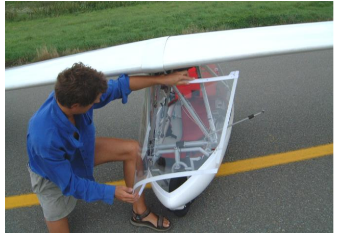
12. Follow the fairing to the nose, and then go on along the fairing.
