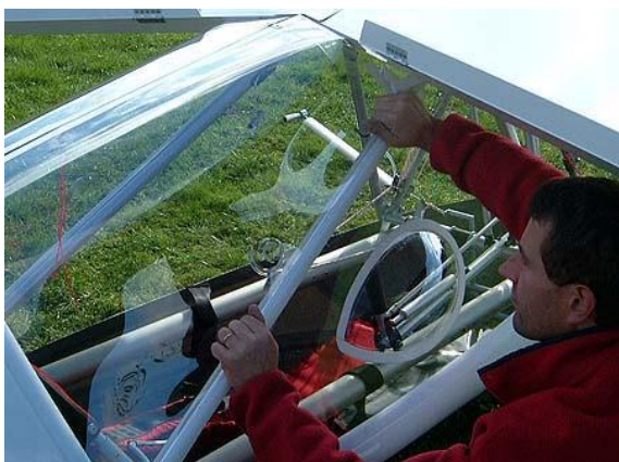
9. Tighten up the Velcro on the oblique tube as well. Then fit the left side window in the same manner.
