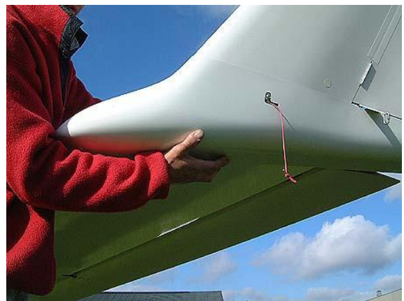
16. Do the same thing on the bottom surface, from the leading edge to the trailing edge one hand on each side of the tip rib.
