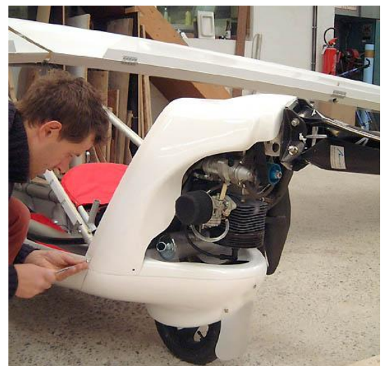
4. Position the engine cover and place the 2 front bolts (button head). The front fairing overlaps the engine cover. Do not tighten the bolts.
