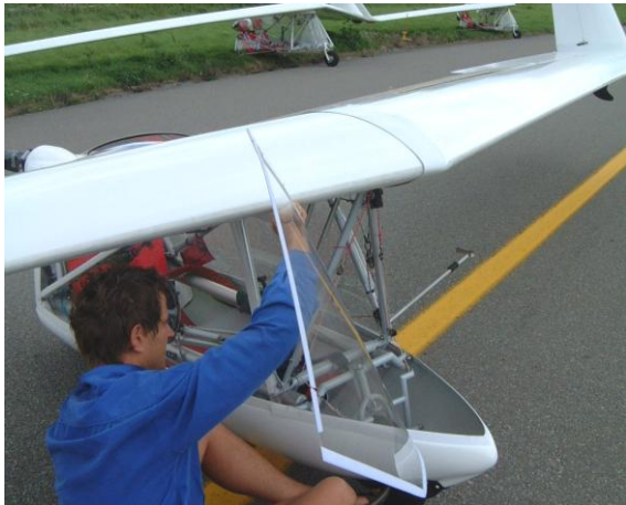
11. Begin from the right edge. Note the position of the lower corner and go on along the vertical tube, pressing firmly the velcro..
