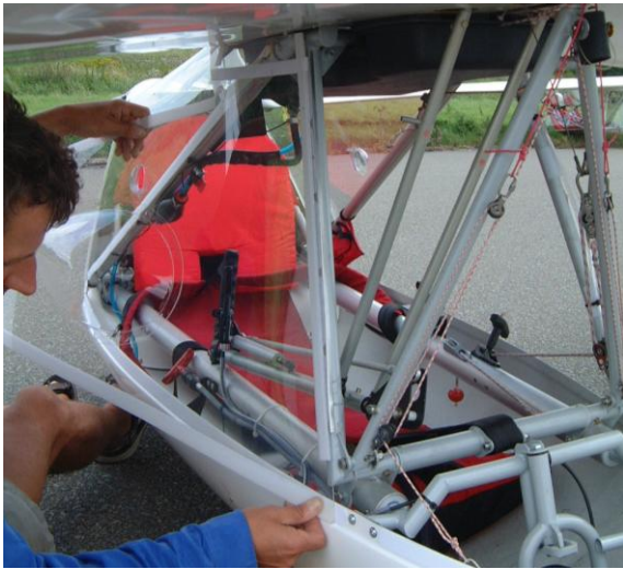
5. Offer up the side window starting with the bottom forward corner following the side tube down.
