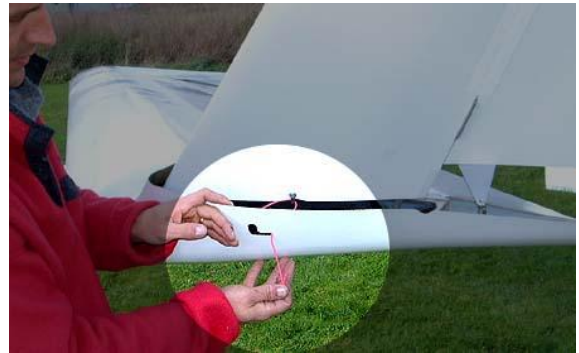
12. Offer up the tip fairing and position. Pass the rudder cable through the little window.
