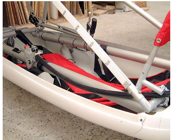
2. Install the engine command group on the main fuselage tube, with a clean routing of the line.
