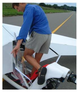
2. Stand up on the Hammock using the trailing edge to balance.
