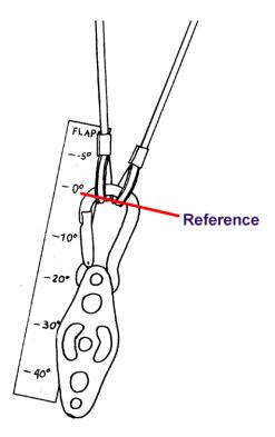
You can control the 0° value of the flaps lining up the elevons and the flaps with the tip fairings (winglets).
