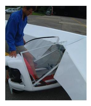
1. Put on the harness. Set the flaps to 40° then from behind put one foot on the hammock (possibly covered with a protection).
