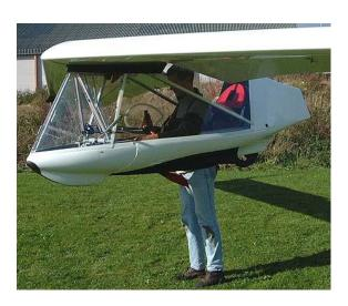
12. Find the pitch balance point with the control stick in neutral by pivoting the glider around your shoulders. Then you can control the wing with the control stick.
