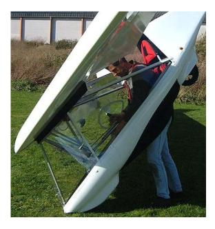
Attach the harness to the parachute bridle find on the right longitudinal tube. Unlock the safety mechanism of the parachute. Adjust the flaps for foot launch (15-20°). Turn on your instruments.
