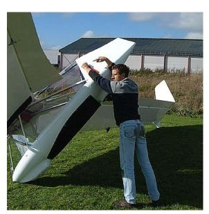
With the **left hand** pulling the strap, lift the tail of the Swift up with the right tiplet<sup>i</sup> pivoting on the ground.
