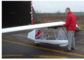
Always support the wing with flat hands, on the bottom surface and on the spar (the spar is in the thickest part of the airfoil) or at the wing tips.
