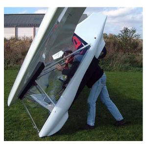
4. Release the lifting handle, which should automatically retract. Put your head, shoulders and left arm insides the trap doors. Put the shoulder straps over your shoulders.
