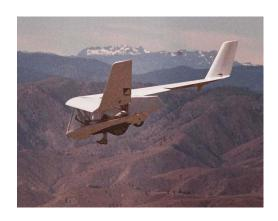
When the pilot is flying in a standing position, the CG position is aft. That is why during T.O. and until the pilot is supine one must keep a bit of forward pressure on the control stick. This peculiarity is a great help during the take off because the elevons facing down together with the flaps increases the lift produce by the wing.
