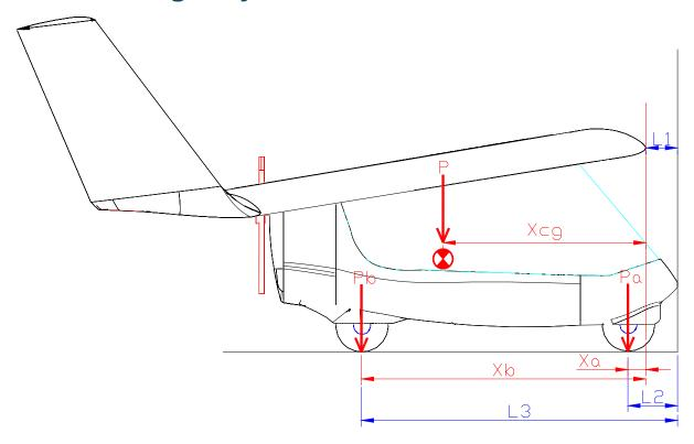
Xcg Horizontal distance of the center of gravity from the nose of the wing
