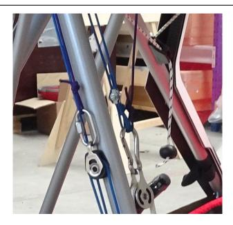
Pull the elevon control rods out through the trailing edge of the wing, pivoting the bellcrank at the root if necessary, then connect the elevon rods between the stick assembly and the wings. A tool with a magnet is provided to facilitate this. Do not connect the elevons to their rods at this stage.
