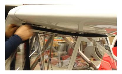
The velcro ends on the fixed frame of the canopy.
