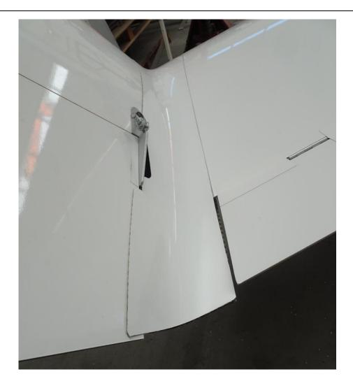
Connect the rudder to the control cable using the quick link.
