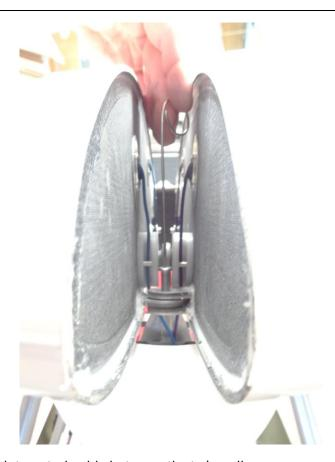
Pass the second winglet control cable between the twin pulleys.
