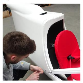
Note: When disassembling the engine cover, do not unscrew the bolt on the back of the cover!
