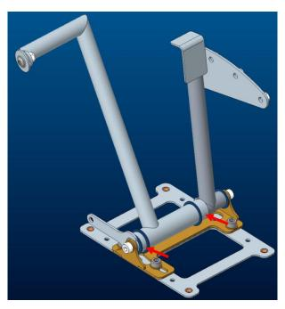
Remove the rudder pedal shaft using the flat wrench provided and change the position of the spacers indicated by the red arrows according to the desired setting.
