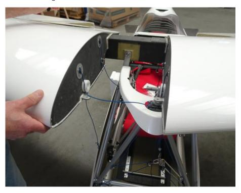
Place the pin securing the 2 wings at the front (the one with a stainless-steel strand making it easier to put in place), and **put the safety ring on immediately**.
