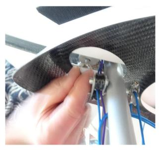
While going around the wing, give a small push to the wing tip towards the rear, to tighten the 2 wings against each other and thus facilitate the installation of the rear axle securing the 2 wings. Put the safety pin in immediately!
