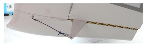
Adjust the trailing edges of the fairing so that it presses lightly against the rudder and has a regular profile towards the elevon, then tighten the velcros.
