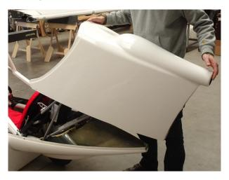
Pass the anti-noise felt in front of the parachute, tilt the hood and ensure that the rear attachment pin is engaged.
