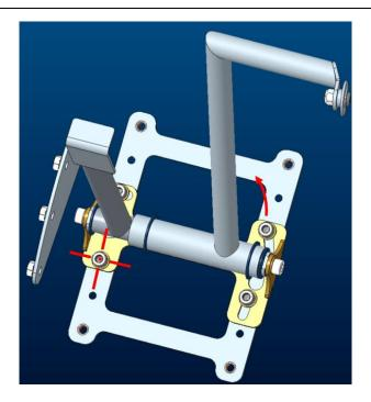
The distance between the pedals can be adjusted by swapping the spacers.
