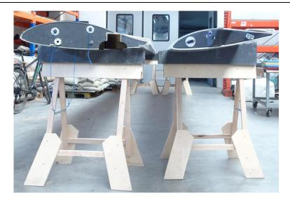
During prolonged storage beyond a few hours (with the wings dismantled), the 2 flap return elastics should be released, even if the flap connecting rods are extended. This is to avoid unnecessary tension on the wing lower skin which could deform them in the long term. See the chapter on assembly.
