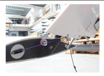
Present the winglet fairing, pass the control cable through the opening and then put the fairing in position on its magnets. The fairing must be engaged in the outer hook.
