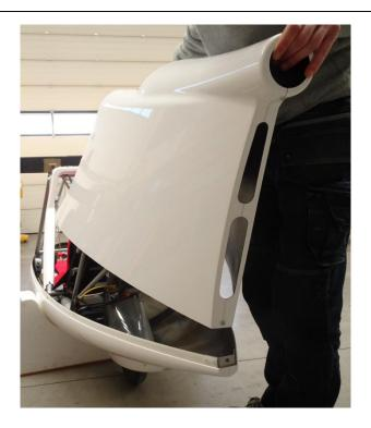
Install the 2 screws securing the cover.
