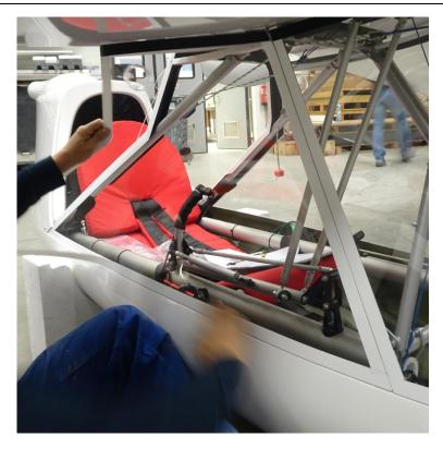
Once the windows are installed, press the velcro fasteners firmly to improve hanging.
