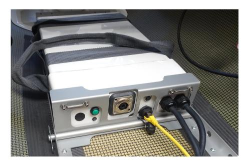
Install the front mounting plate and engage the locking tube from one side to the other. Lock the tube with 2 beta pins.
