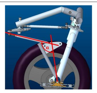
Avoid settings that give an angle that is too flat (= too close to 180°) between the rudder pedals and the corresponding connecting rods, because in this case a little strong pressure on the pedal generates significant forces in the kinematics that can deform the rudder crankbell and lead to the reversal of the kinematics.
