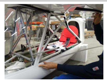
Follow the edge of the windshield on the pillar and fuselage line.
