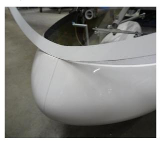
Press the top of the windshield onto the bracket by folding it toward the back of the fuselage.
