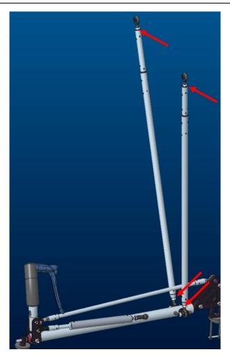
The speed with the stick released for a given flap position can be adjusted by playing with the ball joint of the trim joint, by screwing or unscrewing this ball joint. The ball head can be released by unclipping the plastic head from the ball joint.
