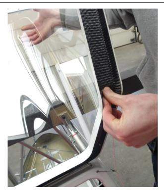
Rotate and remove the hinge pin.
