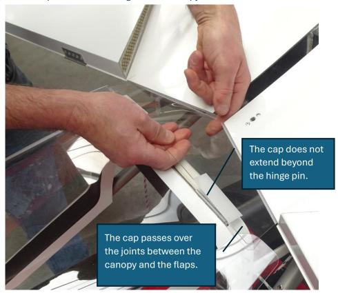
Make sure that the cap is centered on the junction of the wings, that it does not exceed the axis of the hinges (to allow the canopy to open) and passes above the joints between the canopy and the flaps.
