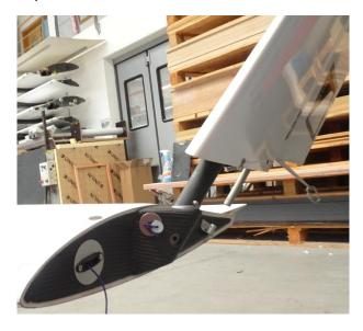
Pass the control cable through the eye strap, but do not connect it at this point.
