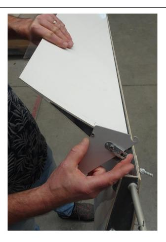
Present the winglet on its support, press the ball in and slide the winglet on its supports until the ball locks. Install the beta pin on the rear bracket.
