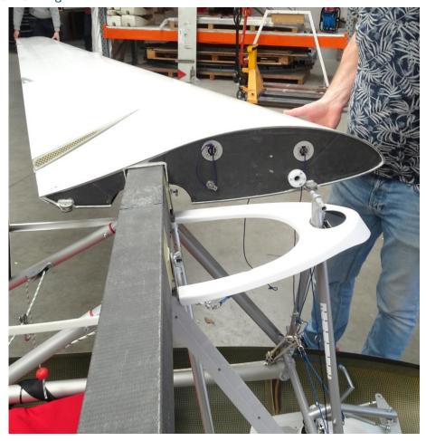
Slide the wing sleeve onto the spar. **Ensure the wing sleeve aligns without forcing** it by matching the wing's height, sweep, and angle of incidence.
