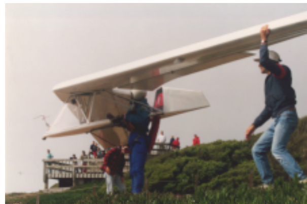
Figure 4. Glider is supported by shoulder straps prior to launch.
