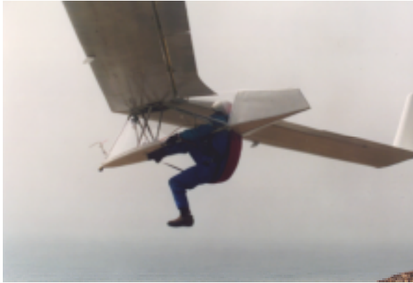
Figure 5. The pilot rotates into flying position supported by a retractable sling.
