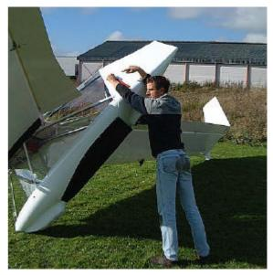
2. With the **left hand** pulling the strap, lift the tail of the Swift up with the right tiplet<sup>i</sup> pivoting on the ground.
