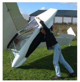
3. Put the **right hand** inside the trap doors, pass **over** the hammock and grab the right longitudinal tube.
