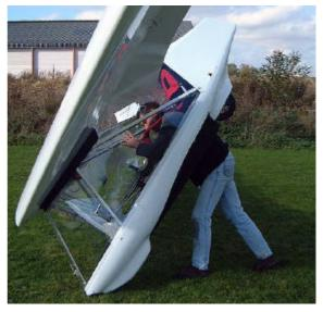
Release the lifting handle, which should automatically retract. Put your head, shoulders and left arm insides the trap doors. Put the shoulder straps over your shoulders.
