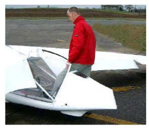
1. Put on the harness. Set the flaps to 40° then from behind put one foot on the hammock (possibly covered with a protection).
