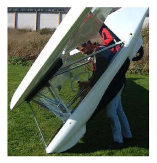
9. Attach the harness to the parachute bridle find on the right longitudinal tube. Unlock the safety mechanism of the parachute. Adjust the flaps for foot launch (15-20°). Turn on your instruments.
