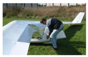
1. Make sure the hammock is in slack position. With the aid of the little strap found on the left hand side of the tail cone, grab this handle by by pulling the lower strand. *If you pull it out holding top and bottom strand it may not retract automatically.*
