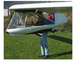
12. Find the pitch balance point **with the control stick in neutral** by pivoting the glider around your shoulders. Then you can control the wing with the control stick.
