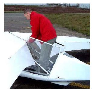
2. Stand up on the Hammock using the trailing edge to balance. **Do not lean on the fairing.**
